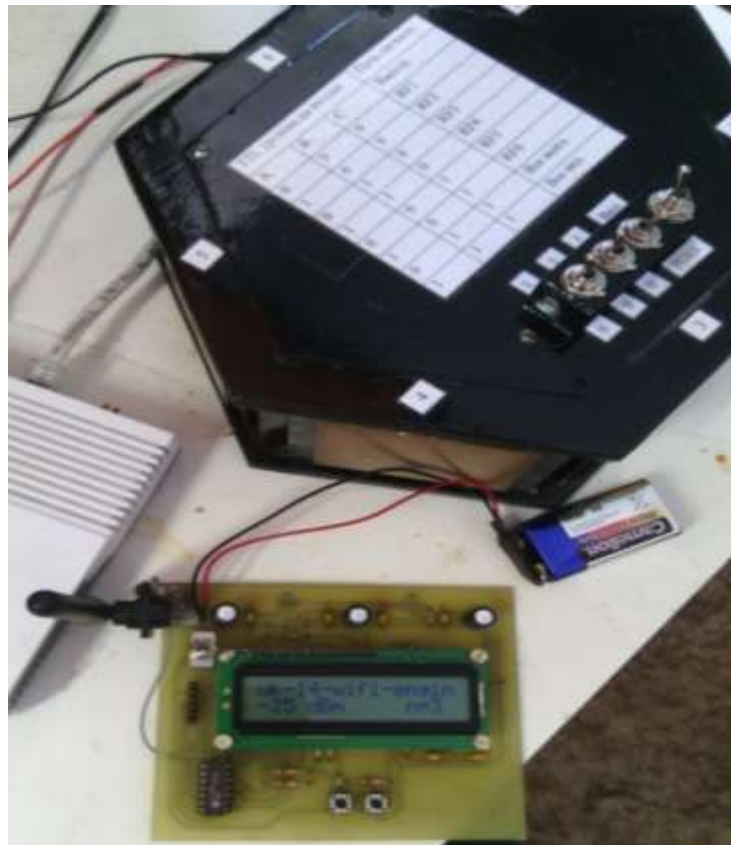
Figure 14. Measuring signal strength on the antenna No. 4.
